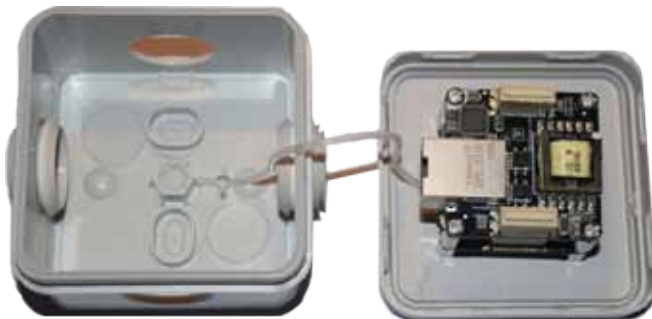
Device Hub - hidden in the ceiling
